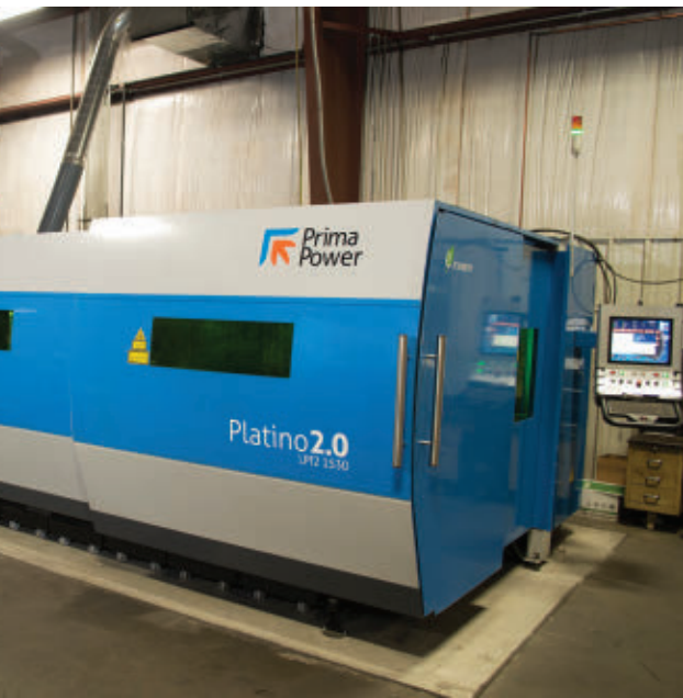
FIGURE 2. The Platino 2.0 fiber laser, with a 10-station tower, cuts a wide range of materials.
