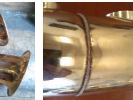
FIGURE 2. Examples of laser-welded sample pieces for saxophones are shown.
