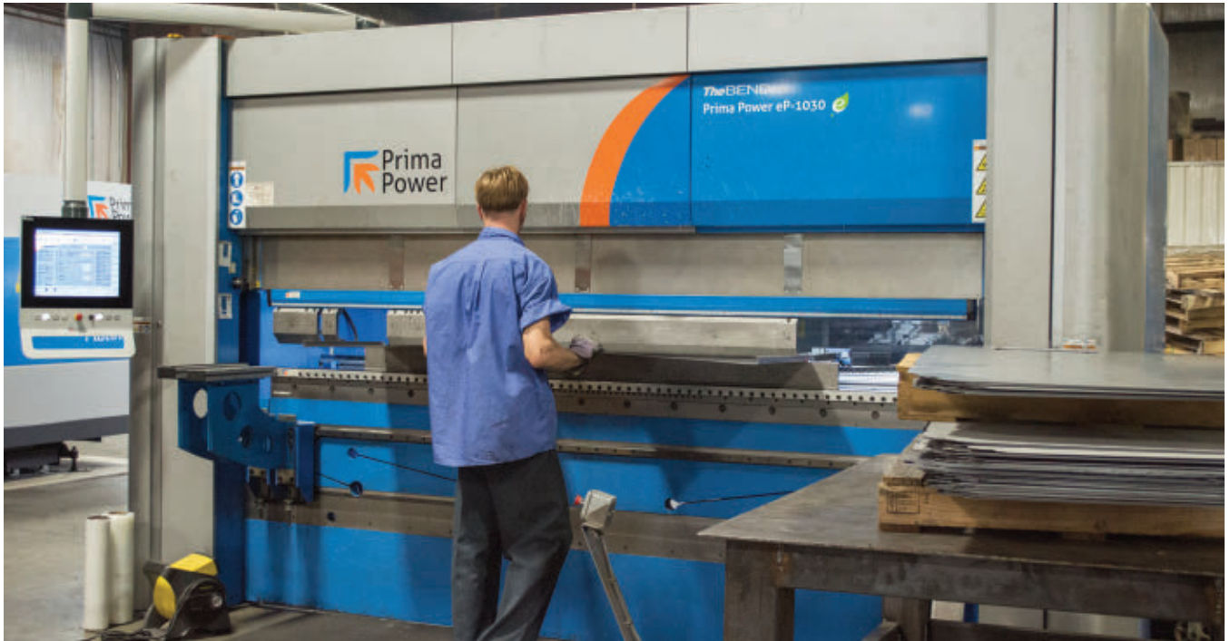
FIGURE 4. The eP servo-electric brake reduces the costs to form metal components by lowering operating costs, increasing productivity, and reducing setup time.
