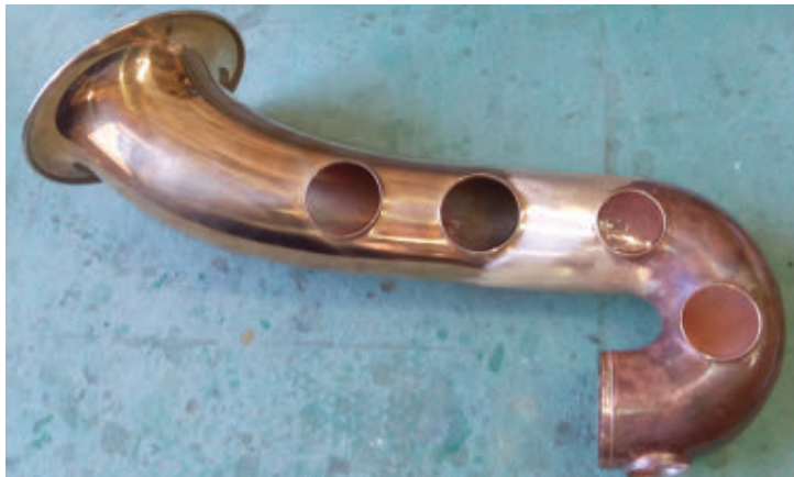
FIGURE 2. Examples of laser-welded sample pieces for saxophones are shown.
