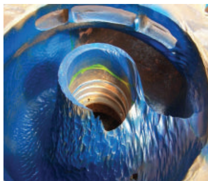
FIGURE 4. A worn refinery slurry pump is shown.
