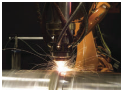
FIGURE 2. A laser-cladding process at work on a truck axle is shown; the process can also be used to repair wind-turbine components, such as damaged or worn shafts.
