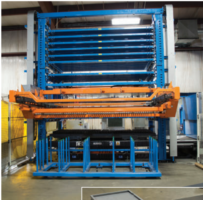
FIGURE 3. The TowerServer allows easy loading/unloading for blanks and processed sheets (inset).
