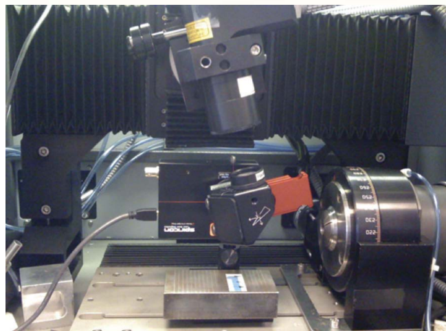
FIGURE 2. Beam profiler on a laser welding system.
