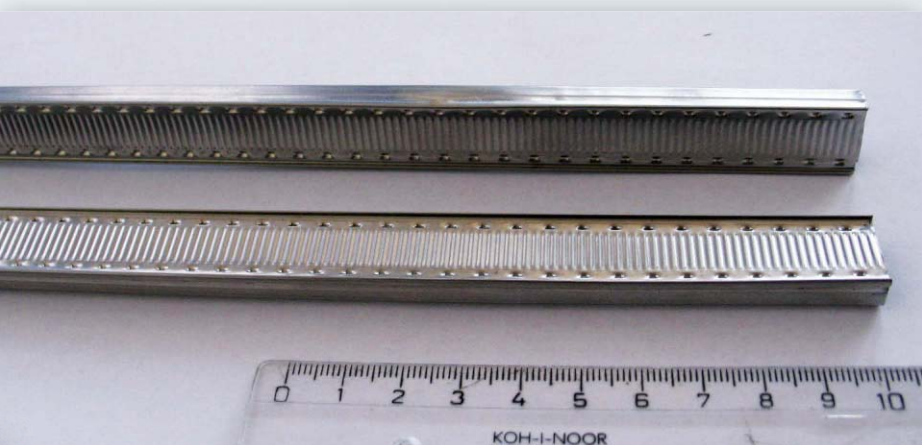
Profile for separating glass plates in windows, welded by a single-mode fiber laser.
