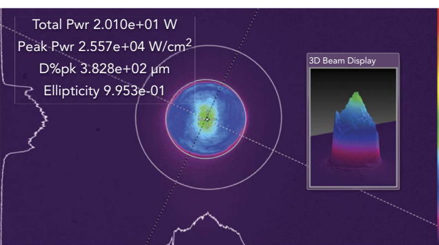
FIGURE 3. Beam profiles on Laser #1 at process parameters: 0.5 kW peak, 9 Hz, 5 ms pulse, and 400 µm spot size.
