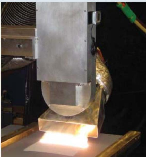
**FIGURE 3.** EWI's polygon scanner has performed a multitude of paint stripping trials using 10kW of fiber laser power, and higher power testing is underway.
