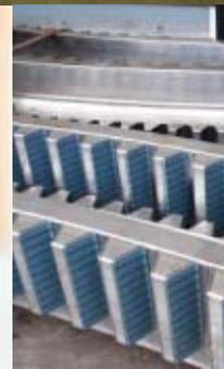
**FIGURE 4. Laserhardened tooth wheel segments.**
