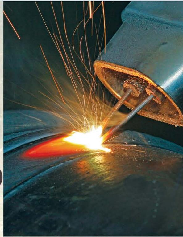
**FIGURE 3.** Dual hot wire laser cladding. Courtesy: Alabama Laser
