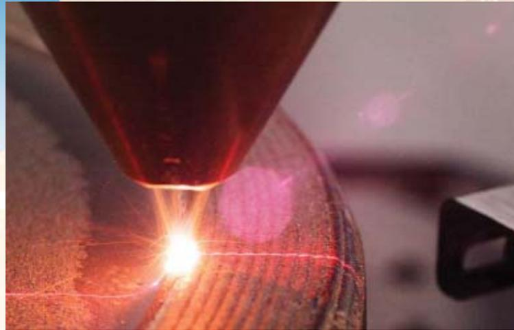
**FIGURE 5.** Example of surface cladding of component face. Courtesy: Joining Technologies
