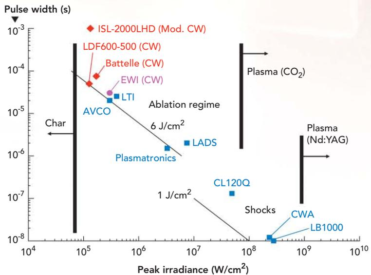
**FIGURE 1.** The substantial range of peak power and interaction times over which laser paint stripping has been accomplished.
