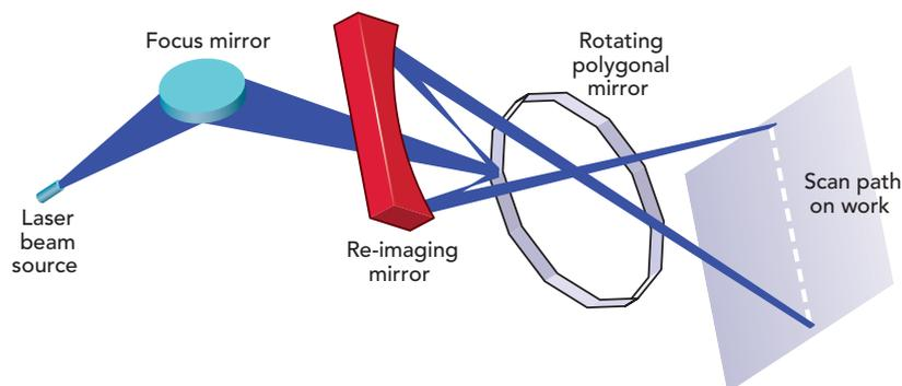
**FIGURE 2.** The fundamental elements of the patent-pending Edison Welding Institute (EWI) scanner design.
