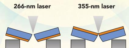
**FIGURE 2.** In LED singulation, a 266 nm (or 355 nm) pulse UV laser is used to scribe through approximately 30% of the total sapphire wafer thickness, followed by mechanical snapping.
