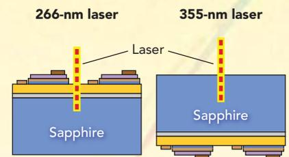
**FIGURE 1.** Bright LEDs are created on a thin sapphire wafer and then separated (singulated) by laser scribing followed by physical snapping with a pressure edge.
