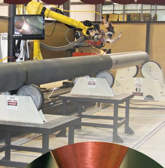
**FIGURE 1.** Large hydraulic road laser clad with powder. Courtesy: Alabama Laser
