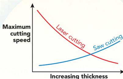
**FIGURE 4.** With so-called low- $\kappa$  materials, mechanical sawing can cause major damage to the integrated circuits.
