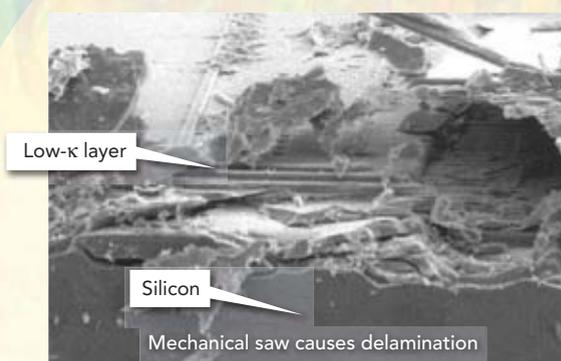
**FIGURE 5.** Chips using low- $\kappa$  materials use laser scribing down the street between the chips. The laser scribes act as crack stops enabling high speed sawing with no damage to the circuitry.
