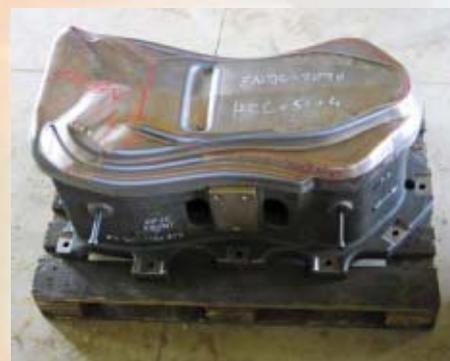
**FIGURE 3. Metal forming tool made of nodular cast iron with hardened edges.**
